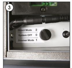
Direct Mode 2: The battery connect directly to illumination. The frame works with %100 bright.
